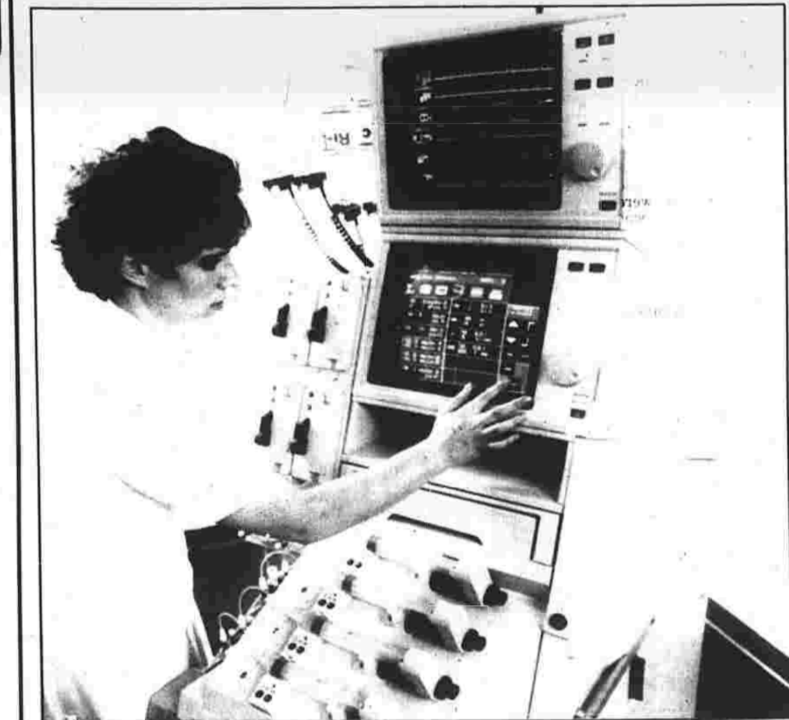
BEDSIDE MANNER - A new monitoring system for hospital intensive care units, which PPG Industries developed jointly with Drägerwerk AG of West Germany was demonstrated Monday in Washington. It is designed to improve patient treatment quality by eliminating a clutter of bedside devices. The prototype displays data on patient's condition, top, simplifies monitoring and therapy control with touchscreen, center, and contains pumps and ventilator.
